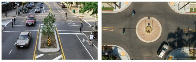
Roadway Reconfigurations typically reduce the number of vehicular travel lanes and may reallocate space to pedestrians and bicyclists and allow room for vehicle turning lanes. Narrower traffic lanes may also contribute to slower speeds while the addition of roadway trees along corridors can have a traffic calming effect.
