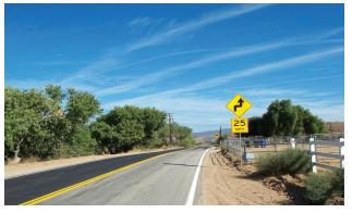
Curve Warning Signs provide emphasis and guidance for a change in horizontal alignment. Advisory speed signs may be used to supplement warning signs.
