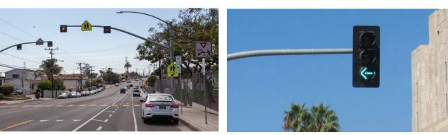
Pedestrian Activated Warning Beacons are flashing yellow lights that provide additional warning to drivers that a pedestrian is crossing the roadway.
